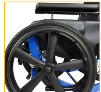
Quick-release mag wheels can be removed for easy transport
