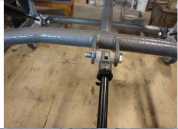
5 Reinstall the 5/16" mounting bolt at the top end of the cylinder.
