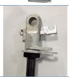
Holding the pin in place screw the cylinder, with cable clip assembly, into the actuator. Make sure the pin stays in place at all times. Tighten the actuator on the cylinder until the pin reaches the top of the hole in the actuator. Do not over tighten.
