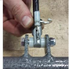
10 Using a 17mm wrench, tighten the black cylinder nut, on the bottom of each cylinder.
