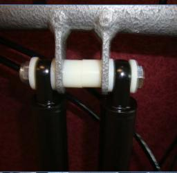
9 Take one 5/16-18 x 3-1/2" long bolt, pass through a #1 spacer, followed by one of the cylinders and a second #1 spacer. Pass the bolt through the first metal tab, followed by two #4 spacers, the second metal tab, followed by a #1 spacers, Second cylinder and a #1 spacer. Secure with a 5/16-18 nylon locking nut. Tighten with 1/2 Wrench.
