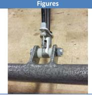
2 Loosen the lock nut located on the stem of the gas cylinder next to the actuator. You will need to wind the stem further into the actuator if the chair is not tilting or reclining, (wind it clockwise) and wind it further out of the actuator if the chair is slowly sliding out of position. (wind it counter-clockwise)
