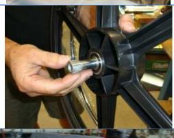
7 Insert a Hex Cap Screw in the appropriate axle hole on the Wheel Mounting Plate. The Hex Cap Screw should be installed from the inside of the frame outwards. Note: If using 14" Mag Wheels, this process must be reversed (i.e. the Hex Cap Screw should be installed from the outside-in).
