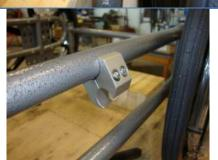
12 Place the wheel lock into the aluminum clamp and adjust so that the splined arm is 1" from the mag wheel when in the unlocked position.
