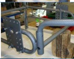
Add a washer per sleeve, before Installing a mag wheel sleeve through the bearing of each Mag Wheel. The large end of the Sleeve should be opposite to the handrims. Set aside until Step 8.
