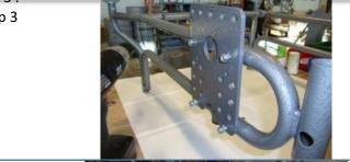
5 Install an anti-tipper into each of the empty caster posts with the small black wheel trailing behind the chair. Secure each antitipper with a hex cap screw, washer then locknut. Tighten fasteners.
