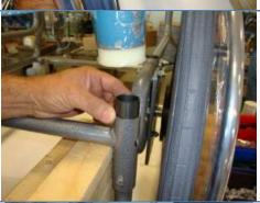
Using a Mallet, tap a 1-1/4" Plug into the top of each rear caster 10 post to cover the exposed end of the tube.
